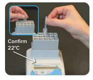
Place tube in Incubator and acclimate for 2 min.\*, then add QuickTox Strip; wait 4 minutes for results.
