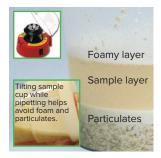
4b. Alternatively, sample may be centrifuged (30 sec) or allowed to settle into layers - avoid foamy layer and particulates when drawing up sample
