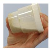
3. Seal/cover container and shake on mechanical shaker (or vigorously by hand) for 30 seconds
