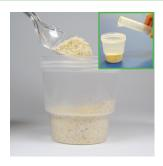
2. Weigh out and add a 20-50 gram sub-sample to container, then add 5 mL/g of water\* (eg: 250 mL for 50g sample)
