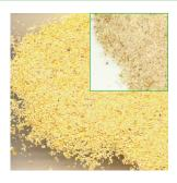
1. Collect and grind representative sample such that ≥95% passes through a 20 mesh sieve
