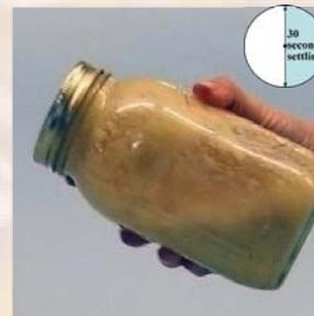
2. Seal container, shake to wet entire sample, settle 30 seconds
