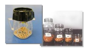
Determine sample weight and grinding method. Weigh sample into an appropriate container.
