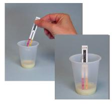
Insert comb or strip into the liquid in the cup. Wait 5 minutes, then read the results, either visually or with QuickScan.
