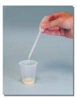
**4.** With pipette, remove 12 mL sample from liquid on top (about 3 pipettefuls, avoid particulates), dispense into a reaction cup. (Note: AS/AQ-050-BGB utilizes a 2 mL reaction vial rather than a cup; fill vial to rim and insert strip.)
